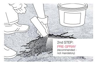
RECOMMENDATION: For maximum durability, we advise that you treat the installation surface with a bituminous primer like **EASYPHALT® PRIME**.
