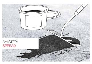
Spread the required amount of EASYPHALT® slightly protruding the height of the original surface.
